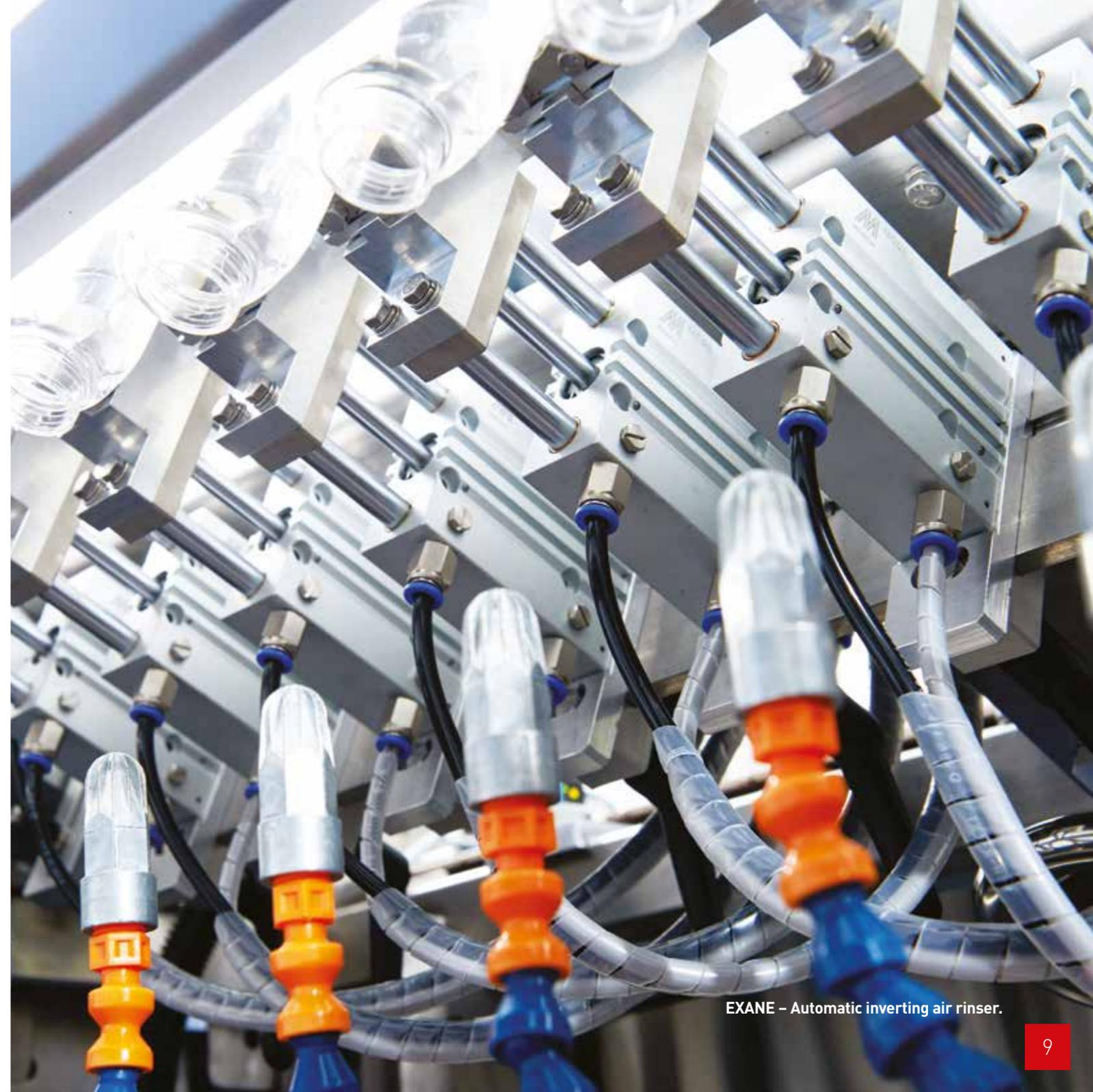
EXANE – Automatic inverting air rinsing.
